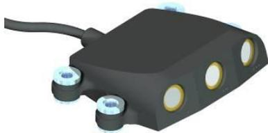
The infra-red sensor measures temperature at a distance without contacting the target. The three channel infra-red sensor incorporates three independent thermopile modules, this enables the spread of temperature across the surface of a tyre to be measured
